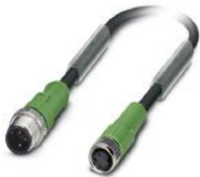
Sensor/actuator cable, 3-position, PVC, black RAL 9005, Plug straight M12, coding: A, on Socket straight M8, cable length: 3 m
