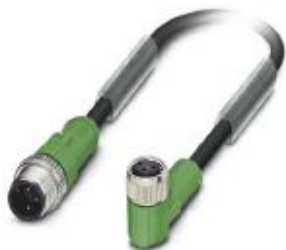
Sensor/actuator cable, 3-position, PVC, black RAL 9005, Plug straight M12, coding: A, on Socket angled M8, cable length: 0.6 m
