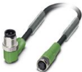
Sensor/actuator cable, 3-position, PVC, black RAL 9005, Plug angled M12, coding: A, on Socket straight M8, cable length: 0.3 m
