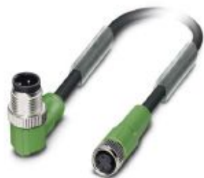
Sensor/actuator cable, 3-position, PVC, black RAL 9005, Plug angled M12, coding: A, on Socket straight M8, cable length: 0.6 m
