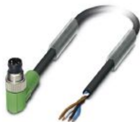
Sensor/actuator cable, 4-position, PVC, black RAL 9005, Plug angled M8, on free cable end, cable length: 1.5 m
