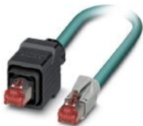
Assembled Ethernet cable, CAT6, shielded, 4-pair, AWG 26 stranded (7-wire), RAL 5021 (water blue), RJ45 plug/IP67 push-pull plastic housing on RJ45 plug/IP20, line, length 5 m
