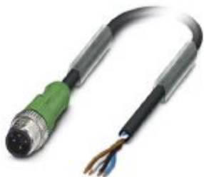
Sensor/actuator cable, 4-position, PVC, black RAL 9005, Plug straight M12, coding: A, on free cable end, cable length: 1.5 m
