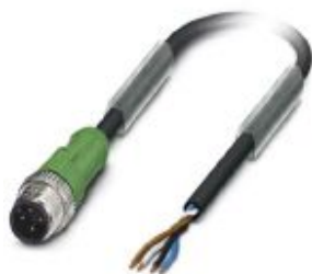
Sensor/actuator cable, 4-position, PVC, black RAL 9005, Plug straight M12, coding: A, on free cable end, cable length: 10 m
