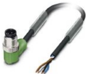
Sensor/actuator cable, 4-position, PVC, black RAL 9005, Plug angled M12, coding: A, on free cable end, cable length: 5 m
