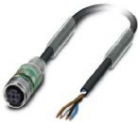
Sensor/actuator cable, 4-position, PVC, black RAL 9005, free cable end, on Socket straight M12, coding: A, with 2 LEDs, cable length: 10 m
