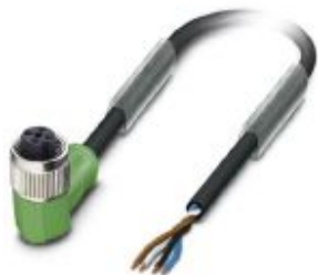
Sensor/actuator cable, 4-position, PVC, black RAL 9005, free cable end, on Socket angled M12, coding: A, cable length: 1.5 m
