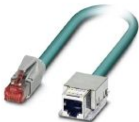
Assembled Ethernet cable, CAT6, shielded, 4-pair, AWG 26 stranded (7-wire), RAL 5021 (water blue), RJ45 socket module/IP20 for Freenet system, 8-pos. on RJ45 plug/IP20, line, length 2 m
