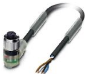
Sensor/actuator cable, 4-position, PVC, black RAL 9005, free cable end, on Socket angled M12, coding: A, with 3 LEDs, cable length: 1.5 m
