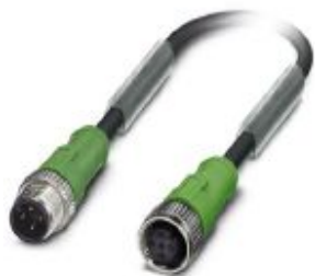
Sensor/actuator cable, 4-position, PVC, black RAL 9005, Plug straight M12, coding: A, on Socket straight M12, coding: A, cable length: 1.5 m
