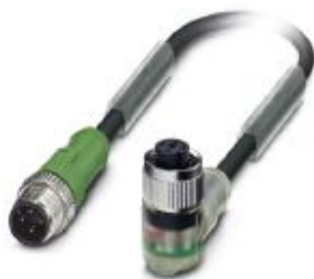
Sensor/actuator cable, 4-position, PVC, black RAL 9005, Plug straight M12, coding: A, on Socket angled M12, coding: A, with 3 LEDs, cable length: 3 m
