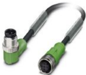
Sensor/actuator cable, 4-position, PVC, black RAL 9005, Plug angled M12, coding: A, on Socket straight M12, coding: A, cable length: 3 m
