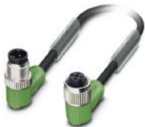
Sensor/actuator cable, 4-position, PVC, black RAL 9005, Plug angled M12, coding: A, on Socket angled M12, coding: A, cable length: 0.6 m
