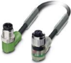
Sensor/actuator cable, 4-position, PVC, black RAL 9005, Plug angled M12, coding: A, on Socket angled M12, coding: A, with 3 LEDs, cable length: 0.3 m
