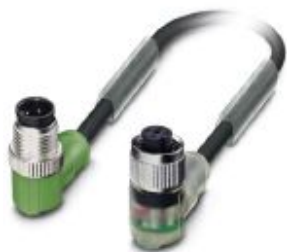
Sensor/actuator cable, 4-position, PVC, black RAL 9005, Plug angled M12, coding: A, on Socket angled M12, coding: A, with 3 LEDs, cable length: 1.5 m
