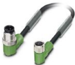
Sensor/actuator cable, 4-position, PVC, black RAL 9005, Plug angled M12, coding: A, on Socket angled M8, cable length: 1.5 m
