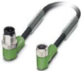
Sensor/actuator cable, 4-position, PVC, black RAL 9005, Plug angled M12, coding: A, on Socket angled M8, cable length: 3 m
