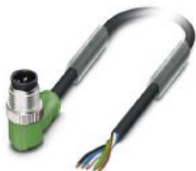
Sensor/actuator cable, 5-position, PVC, black RAL 9005, Plug angled M12, coding: A, on free cable end, cable length: 3 m
