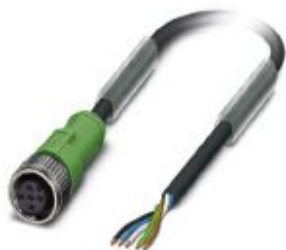
Sensor/actuator cable, 5-position, PVC, black RAL 9005, free cable end, on Socket straight M12, coding: A, cable length: 3 m
