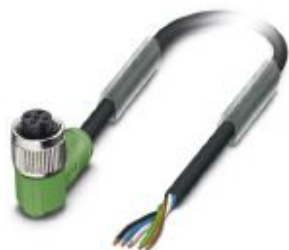
Sensor/actuator cable, 5-position, PVC, black RAL 9005, free cable end, on Socket angled M12, coding: A, cable length: 1.5 m
