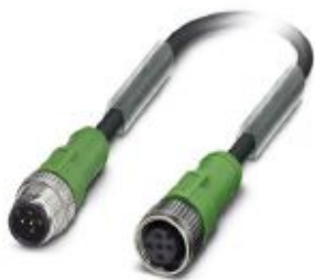
Sensor/actuator cable, 5-position, PVC, black RAL 9005, Plug straight M12, coding: A, on Socket straight M12, coding: A, cable length: 1.5 m
