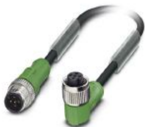
Sensor/actuator cable, 5-position, PVC, black RAL 9005, Plug straight M12, coding: A, on Socket angled M12, coding: A, cable length: 3 m
