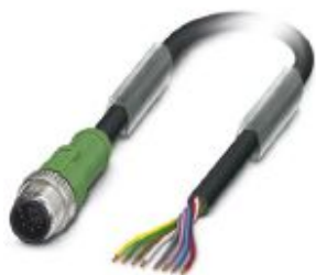
Sensor/actuator cable, 8-position, PVC, black RAL 9005, Plug straight M12, coding: A, on free cable end, cable length: 10 m
