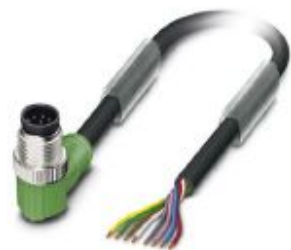
Sensor/actuator cable, 8-position, PVC, black RAL 9005, Plug angled M12, coding: A, on free cable end, cable length: 1.5 m
