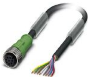
Sensor/actuator cable, 8-position, PVC, black RAL 9005, free cable end, on Socket straight M12, coding: A, cable length: 1.5 m
