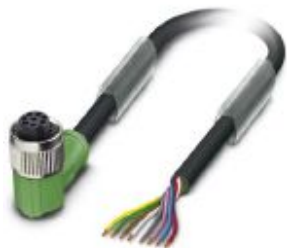
Sensor/actuator cable, 8-position, PVC, black RAL 9005, free cable end, on Socket angled M12, coding: A, cable length: 5 m
