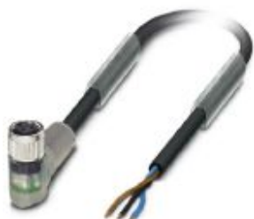
Sensor/actuator cable, 3-position, PVC, black RAL 9005, free cable end, on Socket angled M8, with 2 LEDs, cable length: 3 m
