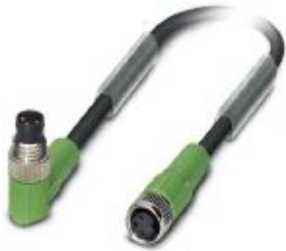
Sensor/actuator cable, 3-position, PVC, black RAL 9005, Plug angled M8, on Socket straight M8, cable length: 1.5 m
