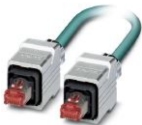
Assembled Ethernet cable, CAT6, shielded, 4-pair, AWG 26 stranded (7-wire), RAL 5021 (water blue), RJ45 plug/IP67 push-pull metal housing on RJ45 plug/IP67 push-pull metal housing, line, length 5 m
