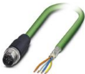
Network cable, PROFINET CAT5 (100 Mbps), 4-position, PUR, green RAL 6018, Plug straight M12, on free cable end, cable length: 2 m
