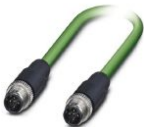
Network cable, PROFINET CAT5 (100 Mbps), 4-position, PUR, green RAL 6018, Plug straight M12, on Plug straight M12, cable length: 2 m
