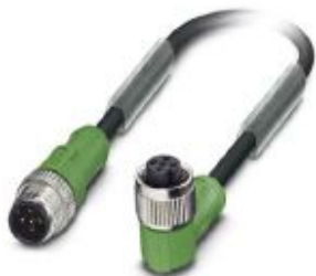
Sensor/actuator cable, 5-position, PUR halogen-free, black-gray RAL 7021, Plug straight M12, coding: A, on Socket angled M12, coding: A, cable length: 10 m
