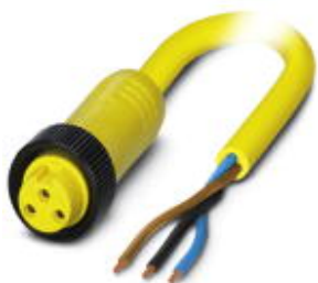
Power cable, 3-position, PVC, yellow, free cable end, on Socket straight 7/8"-16UNF, Cable length: 5 m
