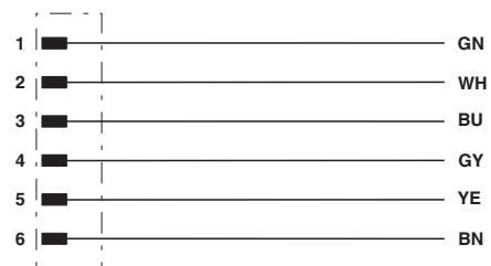
Contact assignment of the 7/8" connector and the 7/8" socket
