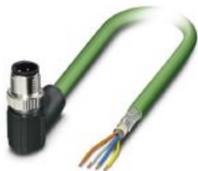
Network cable, PROFINET CAT5 (100 Mbps), 4-position, PUR halogen-free, green RAL 6018, shielded, Plug angled M12 SPEEDCON / IP67, coding: D, on free cable end, cable length: 5 m
