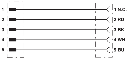
Contact assignment of the 7/8" connector and the 7/8" socket
