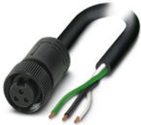
Power cable, 3-position, PVC, black, free cable end, on Socket straight 7/8"-16UNF, Cable length: 2 m
