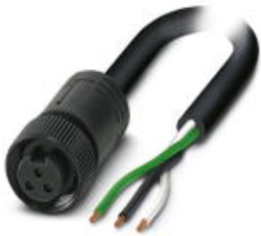
Power cable, 3-position, PVC, black, free cable end, on Socket straight 7/8"-16UNF, Cable length: 10 m
