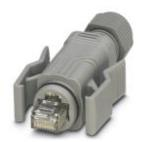
RJ45 connector, IP67, CAT5e, 8-pos., with QUICKON fast connection technology, for 1-wire and 7-wire conductors AWG 26 ... 23, for cable diameter of 5.0 mm ... 8.0 mm, TIA 568 A labeling, color: gray
