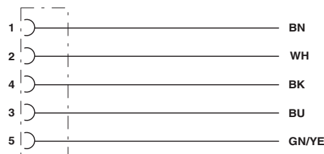
Contact assignment of the M12 sockets
