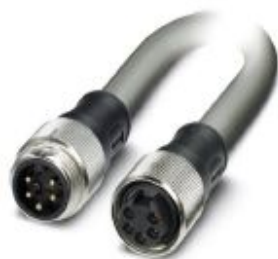
Bus system cable, DeviceNet™, 5-position, PVC, gray RAL 7001, shielded, Plug straight 7/8"-16UNF, on Socket straight 7/8"-16UNF, cable length: 1 m, Connector unshielded
