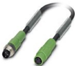
Sensor/actuator cable, 3-position, PUR halogen-free, black-gray RAL 7021, Plug straight M8, on Socket straight M8 Snap-in, cable length: 0.6 m
