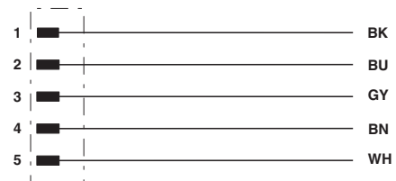
Contact assignment of the 7/8" plug
