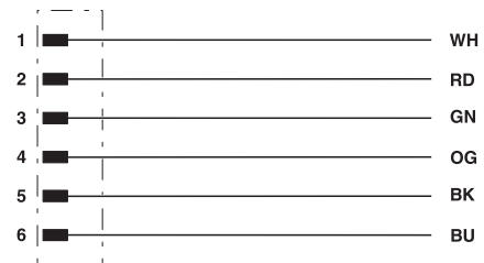
Contact assignment of the 7/8" plug
