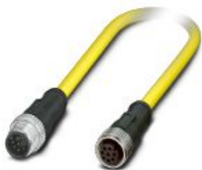
Sensor/actuator cable, 8-position, PVC, yellow, Plug straight M12, coding: A, on Socket straight M12, coding: A, cable length: 3 m
