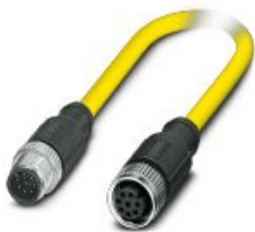
Sensor/actuator cable, 8-position, PVC, yellow, shielded, Plug straight M12, coding: A, on Socket straight M12, coding: A, cable length: 5 m
